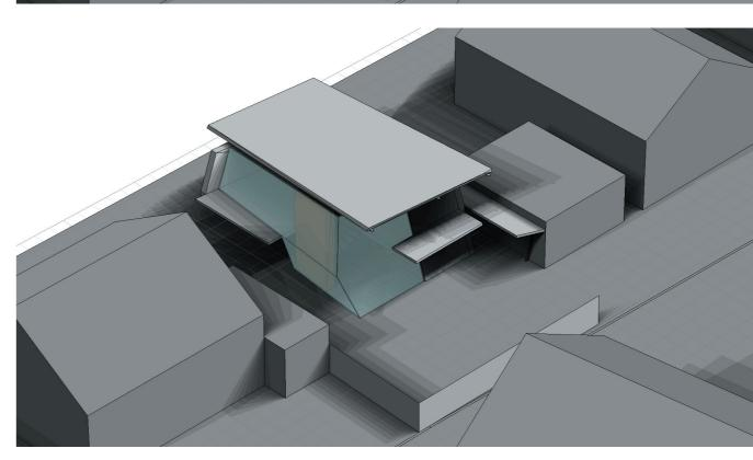
Designation of zones with maximal sun exposure (coloured) and adaptive building design (grey) coupled with with shadow analysis. Simulations using EcoTect . Computer generated images (CGI)
